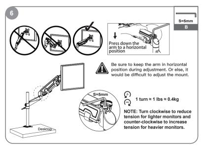
Use a 5mm hex wrench to adjust the height tension of the gas spring arm, to keep different weight of monitors still at any position.
