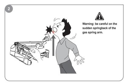
Tear off the cable tie and rebound carefully.
