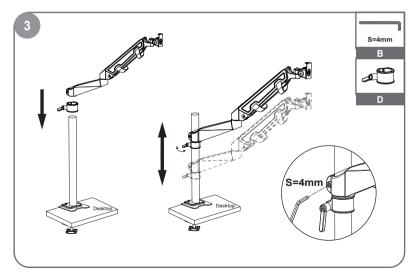
Insert the arms to the steel pipe above the locating ring.
