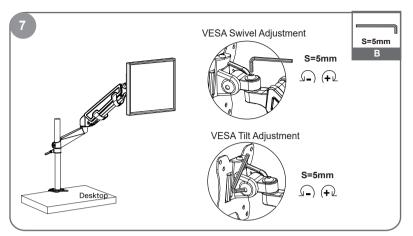
Use a 5mm hex wrench to adjust the damp for Tilt and Swivel. Turn counter-clockwise to reduce damping and clockwise to increase damping.
