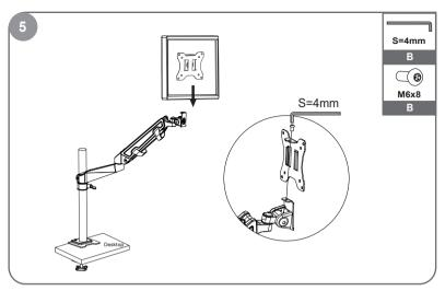
Insert the monitor along with the VESA plate to the arm and lock it.
